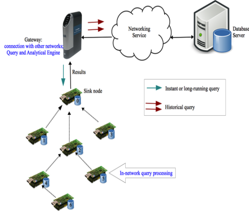
Fig. 2. Illustration of a distributed database architecture for wireless sensor networks.
